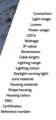
Driving beam 4.920 lumen 42 Watt IP69K 100cm cable 1 lux at 315m White / amber Not included Polycarbonate Aluminium Light bar Black ECE-R10
